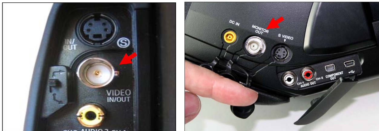
Example of the BNC Video out on a Canon XL2 and a Sony PMW-EX3 Video Camera.
